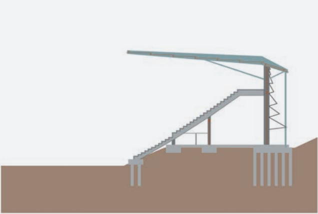
4. Installation of roof structure and completion of construction phase 2
